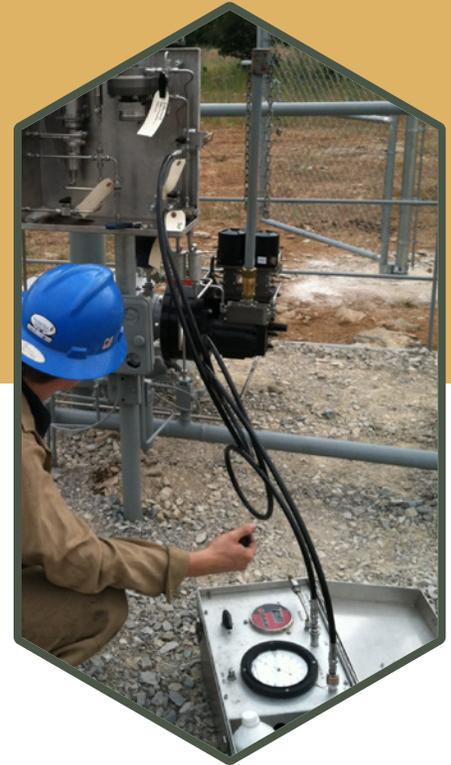
ATI technicians are experienced in the use of calibration test kits in order to keep field instrumentation accurate and problem-free. We can conduct field calibration on safety systems in the field with our proven rate-of-drop test kits. If preferred, we can supply the kits and training for your personnel. Either way, we are your partner in providing safe pipeline control.
